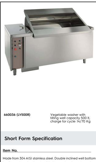
to allow automatic cleaning. Washing system by water vortex; multiple diffuser for uniform water vortex; automatic water filling. The lifting of the basket at the end of the washing cycle is achieved by a reliable and safe linear motor controlled by double push button with alarm. IP55 water protection. Well capacity: 500 It. Load per cycle: 14 kg (light vegetables); 70 kg (heavy vegetables). Cycle duration: 2-3 min.
